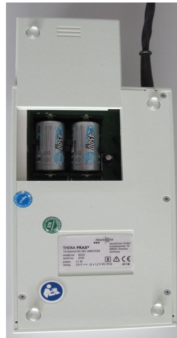
batteries in the battery compartment
