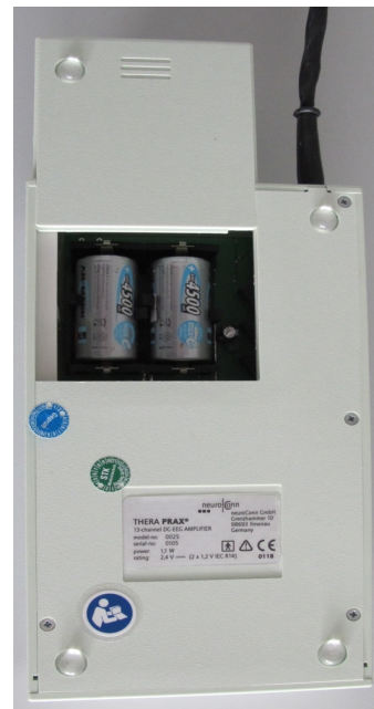
batteries in the battery compartment
